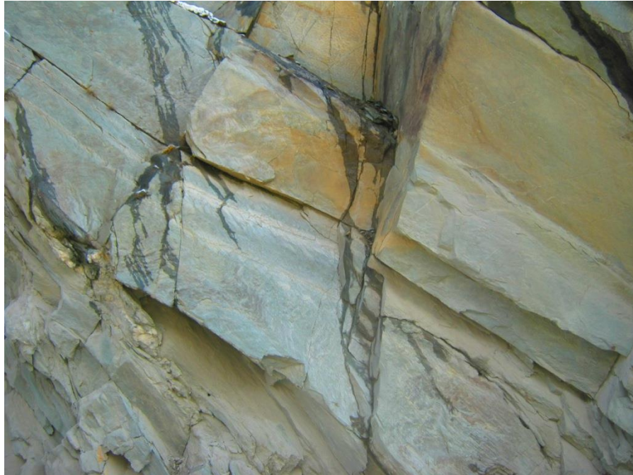
Fig.38 A View of joint sets in Basic rock
