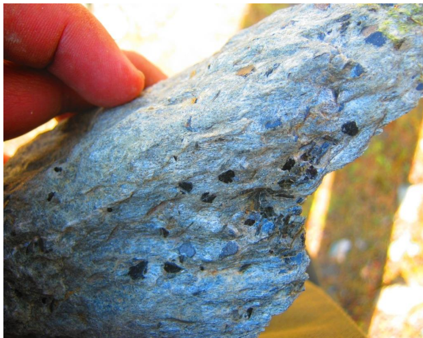
Fig. 29 A close View of Fine grained Porphyroblastic Panjal Trap rock
