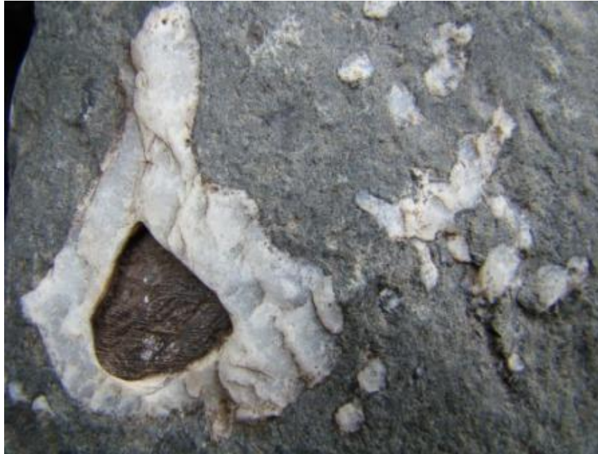
Fig. 32 A View of Vesicular basic rocks, Vesicles filled by Secondary minerals.
