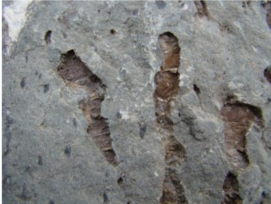
Fig. 30 A Close View of Vesicular structure in fine grained basic rocks.
