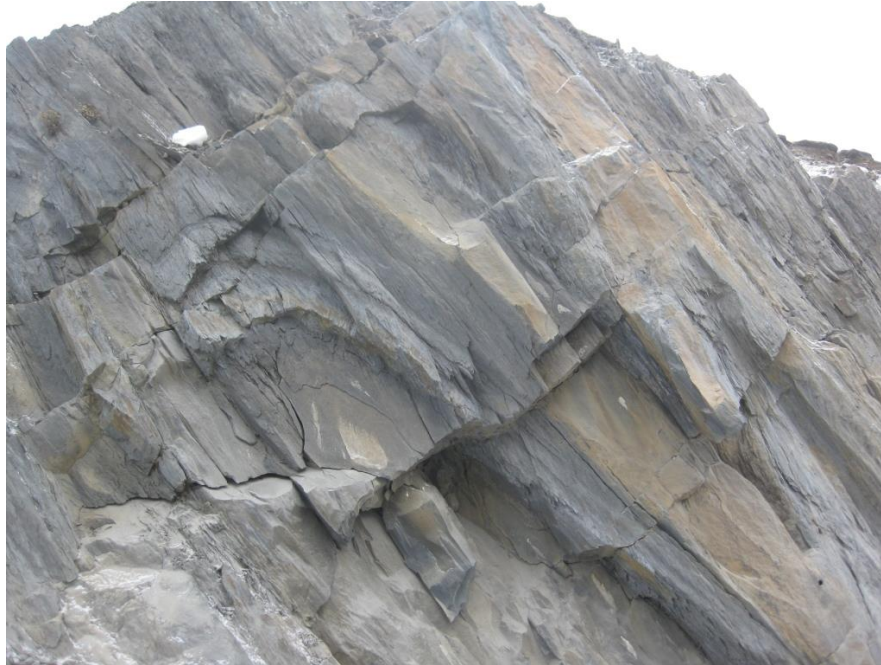
Fig. 27 A View of Zoji-La formation having steep foliation and three set of joints.
